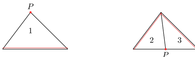
Figure 6: Stage 1: Original triangle(left) in congruence class 1 Stage 2: Applied the newest vertex bisection once(right) in congruence class 2 and 3.
